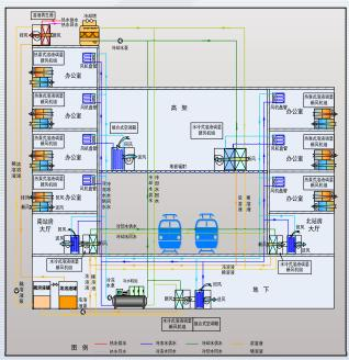
Operational state of air-conditioning system with independent control of temperature & humidity at Tianjin Railway Station in summe
